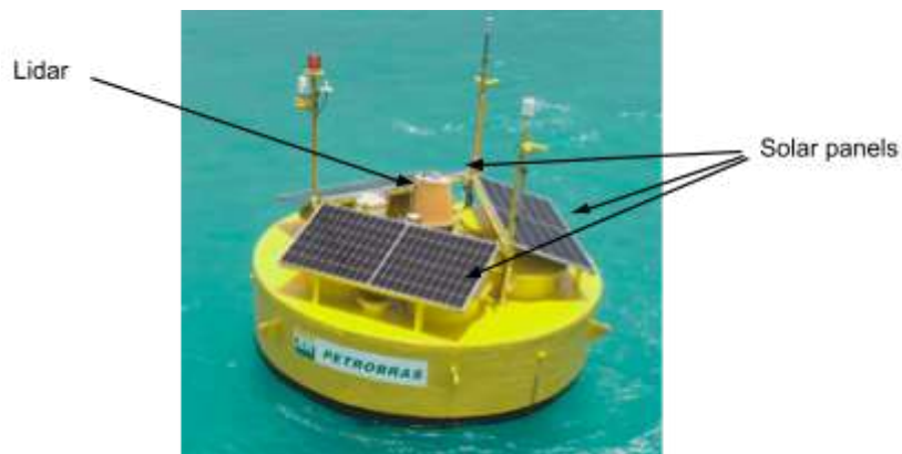
Figure 2: General view of the Bravo Buoy, developed by Petrobras and the SENAI Institutes of Innovation in Renewable Energies (ISI-ER) and Embedded Systems (ISI-SE).
